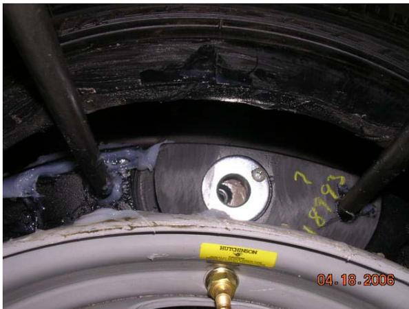
5. Install the two mounting bars in the installation holes located at the end of each side of the CRF arcs. See the previous photo.
