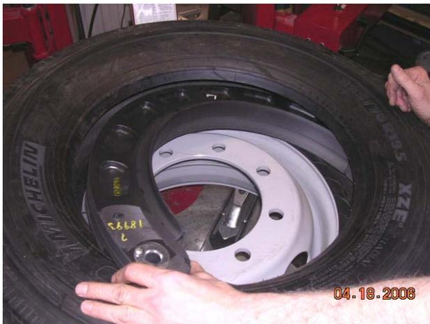
3. Lubricate the bottom bead and mount the bottom bead on the tire leaving the top bead outside the wheel flange. The CRF should fall into the tire when the bead is seated. If the CRF does not fall into the tire, push the CRF at the connected portion with a tire iron until it falls into the tire.
