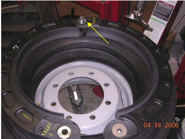
2. Snake the roller halves into the tire as shown in the following photo
