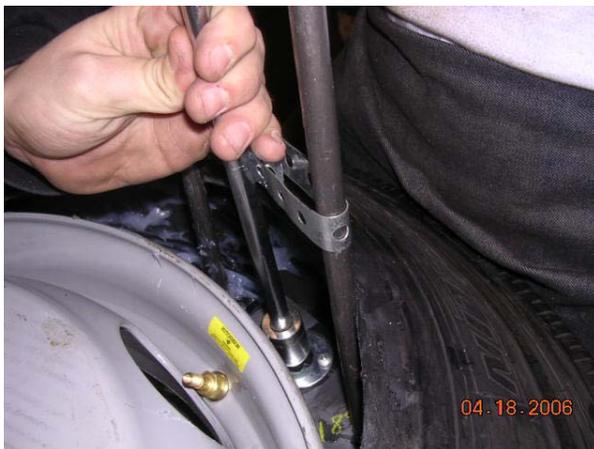
8. Loosen the safety clip mounting screw and install the bolt safety clip over the nut. Secure the mounting screw.
