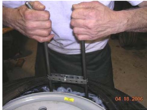
7. Continue to tighten the bolt down until the bolt is secure to 30 ft lbs.
