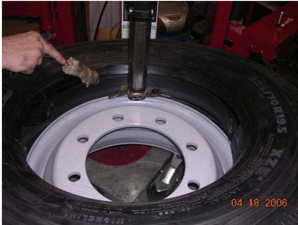
4. Once the bottom bead is seated, locate the open end of the CRF inside the tire and move the CRF so the open end of the arcs is located at the valve hole location. You may use the installation bars or tire iron to move the CRF to the proper location. See the following photo.
